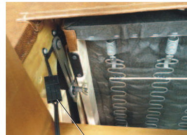
Thermo-Electric Cooler Power Transformer Connection
