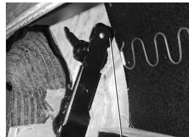
Back and Body Brackets Engaged
